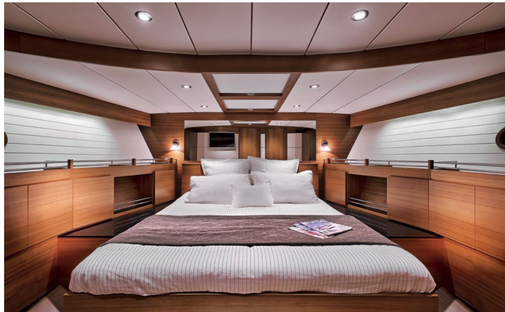
OWNER'S CABIN WITH A KING SIZE BED. ALL WOODWORK IN LIGHTWEIGHT FOAM CONSTRUCTION WITH TEAK VENEER.
